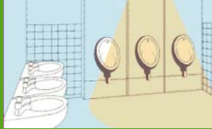
PIR Controlled Urinals
