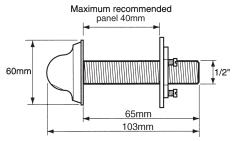
**Panel Mounted** (suitable for panels up to 40mm thick)
