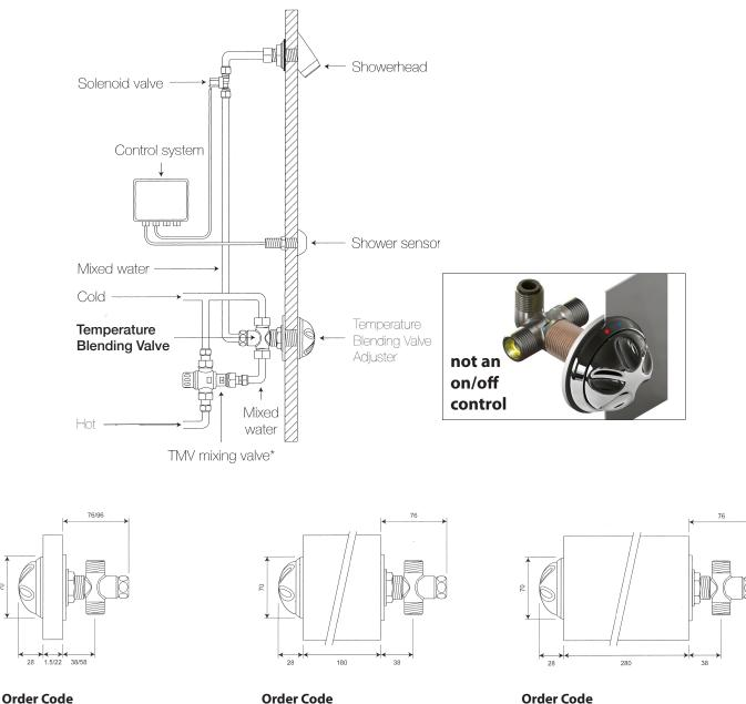
**Order Code** TBV/ADJ/180 Application For up to 180mm wall thickness. Fixing ¾" BSP. (Ø28mm drill hole)
