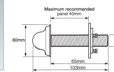
**Panel Mounted** (suitable for panels up to 40mm thick)
