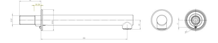
Spout with 90 degree water outlet with integral 5 Lpm flow regulator
