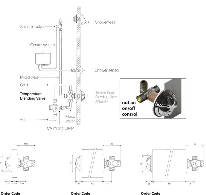
Order Code TBV/ADJ/180 Application For up to 180mm wall thickness. Fixing ¾" BSP. (Ø28mm drill hole) Order Code TBV/ADJ/280 Application For up to 280mm wall thickness. Fixing ¾" BSP. (Ø28mm drill hole)
