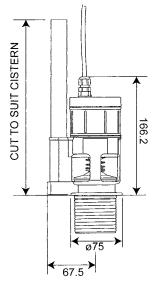
c/w 1<sup>1</sup>/<sub>2</sub>" standard down-pipe connections so it can easily be fitted into new or existing UK industry standard flat bottomed cisterns and flushing troughs. Valve c/w internal overflow pipe.
