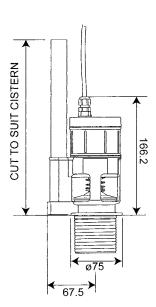
c/w 1½" standard down-pipe connections so it can easily be fitted into new or existing UK industry standard flat bottomed cisterns and flushing troughs. Valve c/w internal overflow pipe.
