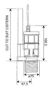
c/w 1<sup>1</sup>/<sub>2</sub>" standard down-pipe connections so it can easily be fitted into new or existing UK industry standard flat bottomed cisterns and flushing troughs. Valve c/w internal overflow pipe.
