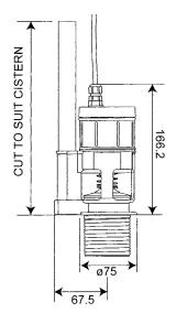
c/w 1½" standard down-pipe connections so it can easily be fitted into new or existing UK industry standard flat bottomed cisterns and flushing troughs. Valve c/w internal overflow pipe.
