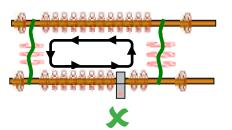
This is an electrical loop, the signal does not propagate correctly and is trapped in the loop By moving the unit to a different location, out of the loop, the signal propagates throughout the system.
