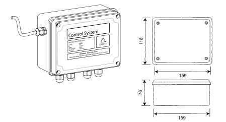
**Battery Bath Control Box:** with adjustable valve open time from 1 minute to 10 minutes.
