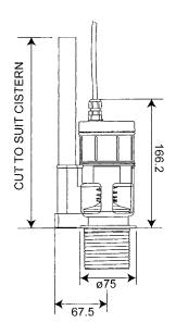
c/w 1½" standard down-pipe connections so it can easily be fitted into new or existing UK industry standard flat bottomed cisterns and flushing troughs. Valve c/w internal overflow pipe.
