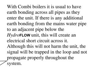
By moving the unit below the cross bonding, the short circuit is removed and the signal will then propagate correctly throughout the system.
