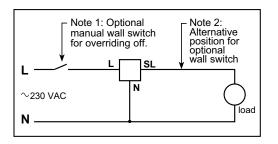
Wiring diagram: Multiple presence detectors
