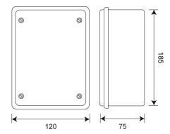
Electrical supply: 9v DC from 6 x 'C'-cell battery pack. Amps: 0.14A (max.) Control box dimensions: 120mm (w) x 185mm (h) x 75mm (d) Control box weight: 1kg
