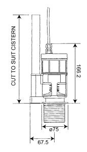
2" base connection for compatibility with our flat bottomed cisterns c/w 2" flush pipe. Valve c/w internal overflow pipe.
